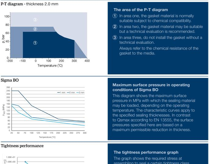
The graph shows the required stress at assembling to seal a certain tightness class. The determination of the graph is based on EN13555 test procedure which applies 40bar Helium at room temperature. The sloping curve indicates the ability of the gasket to increase tightness with raising gasket stress.
